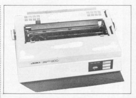
printer because of the mechanicals involved and the sheer force needed to thump a solid letter on a daisywheel stalk against the ribbon and on to the paper.
