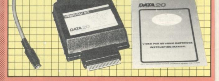
the 64). A short video lead which plugs into the monitor output to enable the system to display the standard CBM screen when the cartridge is not activated. There are two five-pin DIN sockets in the rear of the cartridge; the first takes the other end of the video lead, the second is where you plug in your monitor.
